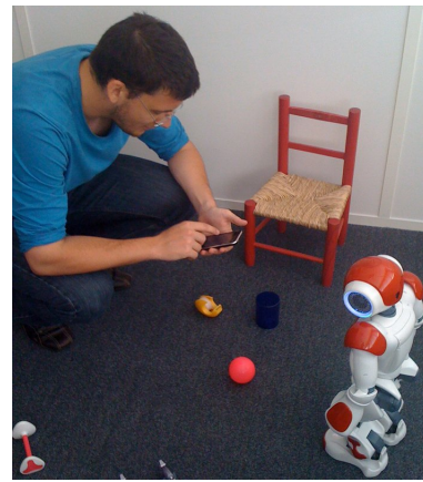
Fig. 1. Using a handheld device as a mediator object to control the movements of a social robot.
