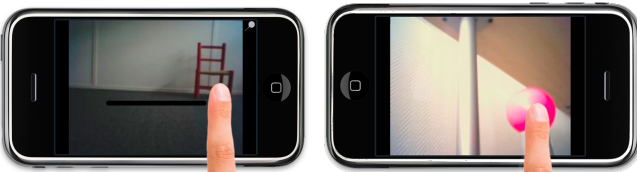
Fig. 3. Drawing attention towards an object: the user first sketches directions to position the robot such that the object is in its field of view (left), and if he wants to center the robot's sight on a specific spot just past on it (right).
