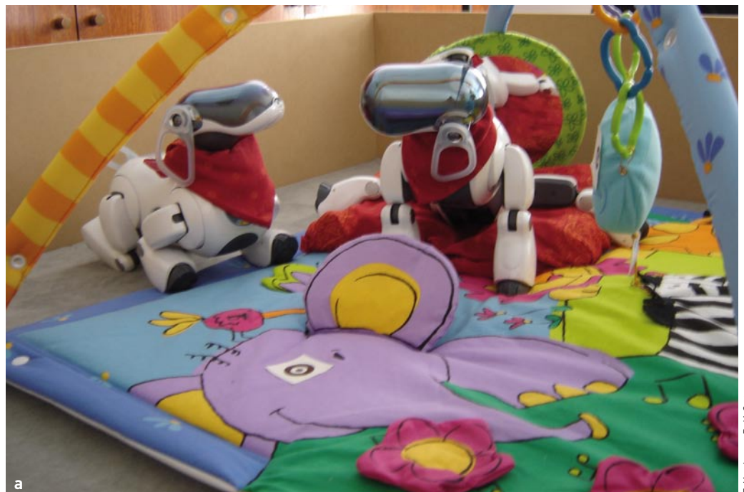
The AIBO robot, developed by Sony, is used by scientists to study how a system of curiosity may enable it to learn about its environment on its own (a) and what the mechanisms are that enable it to learn the names of objects tested in interactions with humans (b).
